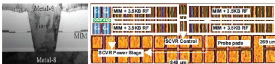
Cross-sectional TEM image of MIM capacitor and die photo.
